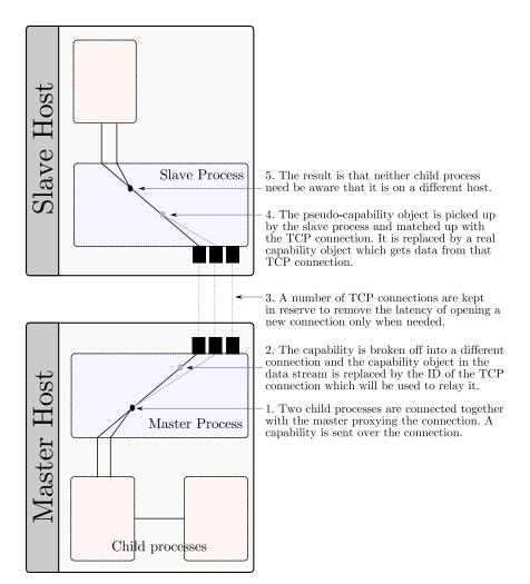
Figure 6.1: Transparent handling of capabilities across hosts
