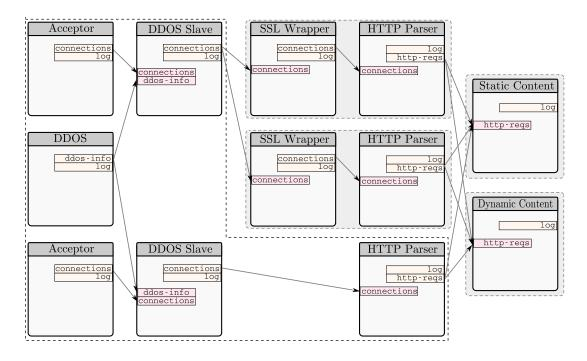
Figure 7.2: A more complex capability deconstruction of an HTTP server
