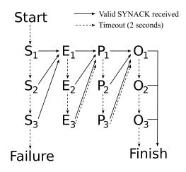
Figure 1: Prober state machine
